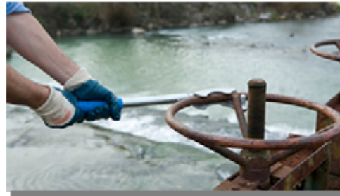
Image 7 and 8 The tool allows the opening and closing of vertical and horizontal fly valves.
