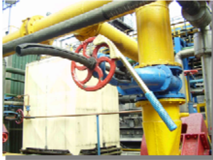
Image 7 and 8 The tool allows the opening and closing of vertical and horizontal fly valves.
