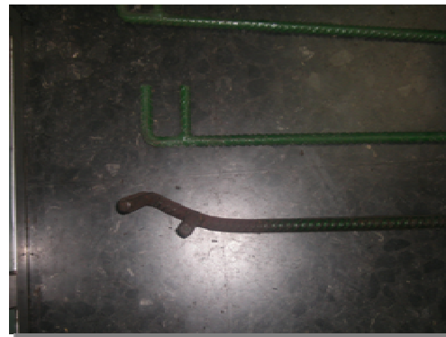
Image 2 Tool bent due to fatigue.
